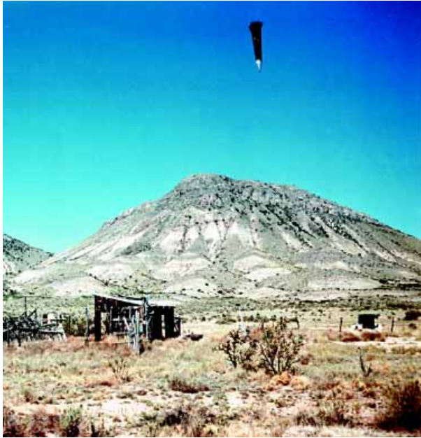
Figure 4. PII reentry vehicle nearing impact in a shot at White Sands Missile Range. The actual target was the corner of the building closest to the flight path of the reentry vehicle.
